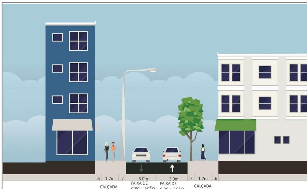
Figura 44: Corte Tipo – Via Local
